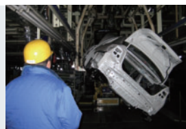
A car body shaken loose from an overhead clamp (Yajima Plant)
